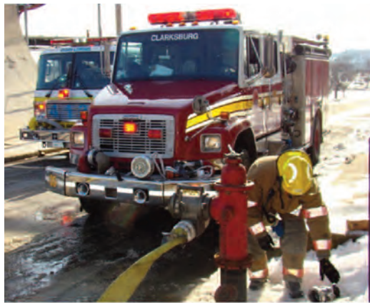
Figure 16: Connecting to the Hydrant
