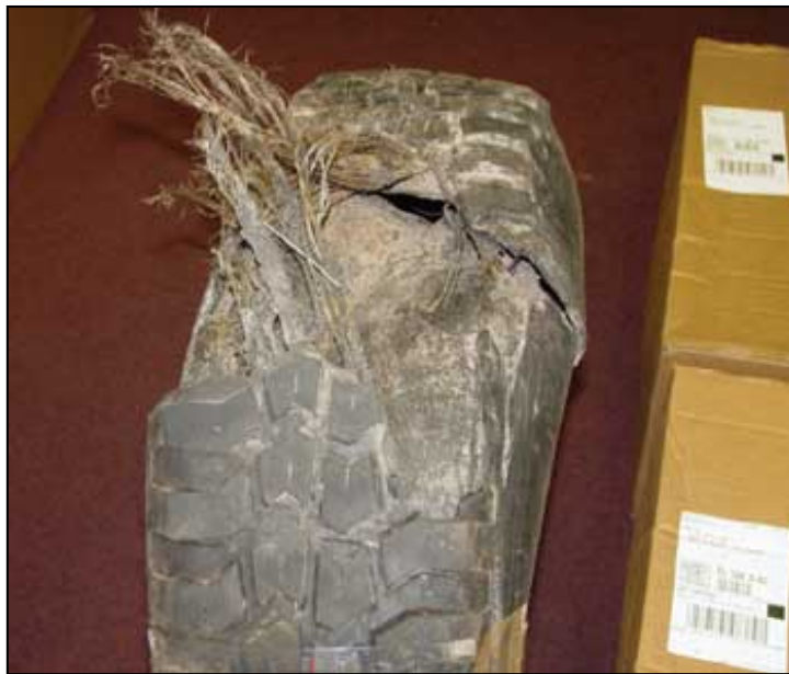
Photo. Right front tire after blow-out.
