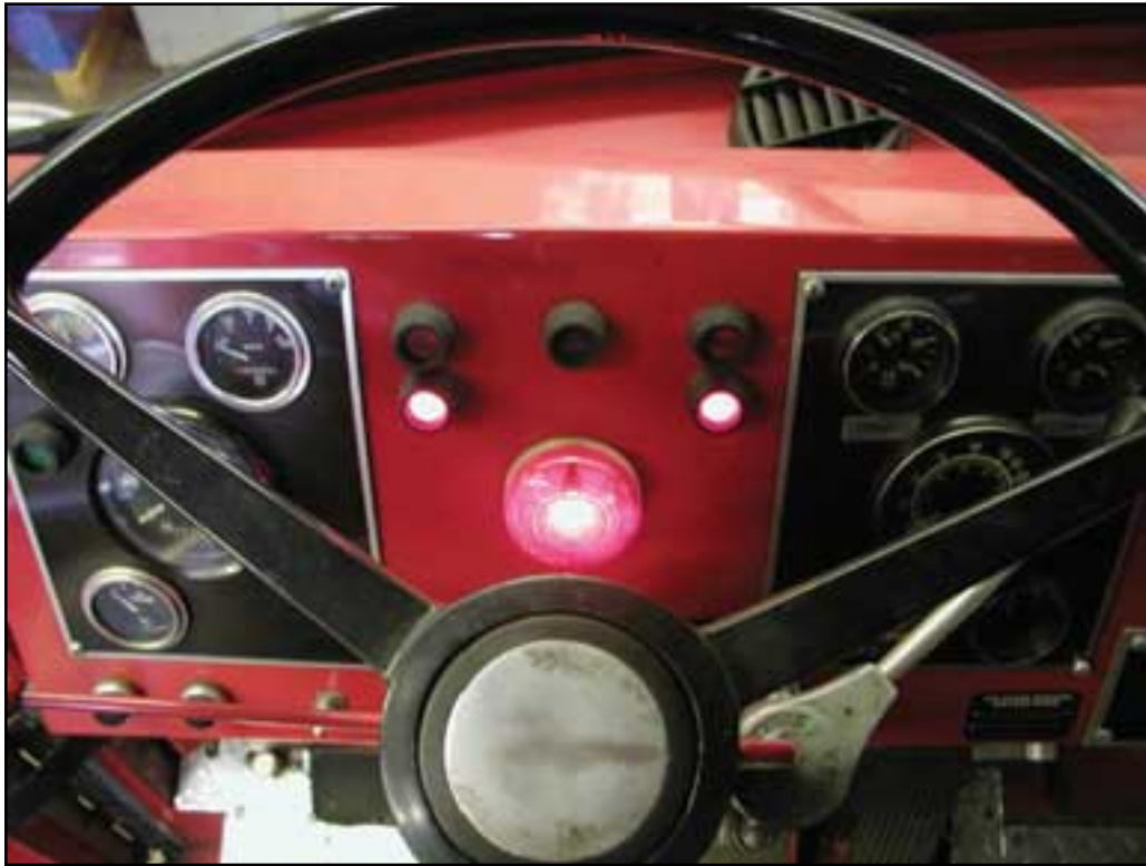
Photo 4. Red light on dash that flashes when the electronic signal button is pushed
