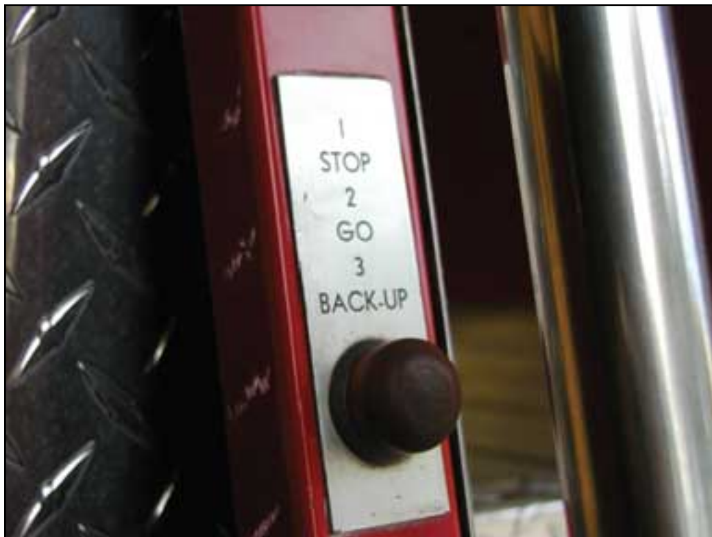
Photo 3. Push button on rear panel of engine with operating instructions
