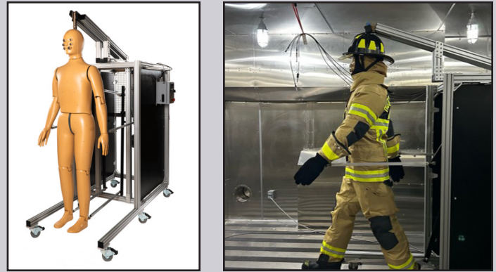
Figure X. "Andi" Physiological Manikin at Florida State University Equipment (left) and with Turnout Gear During Test (right)
