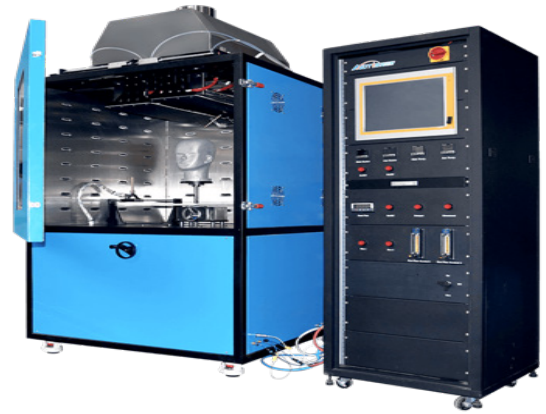
Equipment used to measure heat resistance of helmets, gloves, boots, hoods, and garment materials
