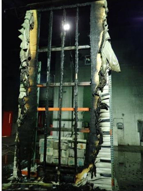
Figure 45 - Post-test Photograph of Test 6 Vinyl Siding/House Wrap/Plywood Wall Assembly with 100 kW Ignition
