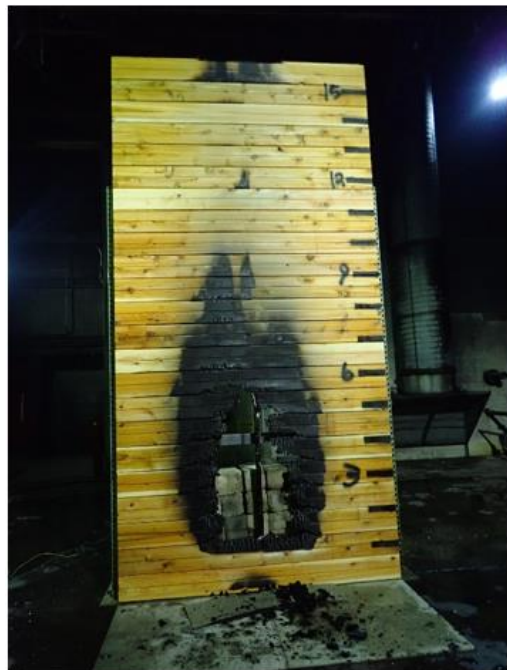
Figure 44 - Post-test Photograph of Test 5 Cedar Siding/House Wrap/Plywood Wall Assembly with 100 kW Ignition
