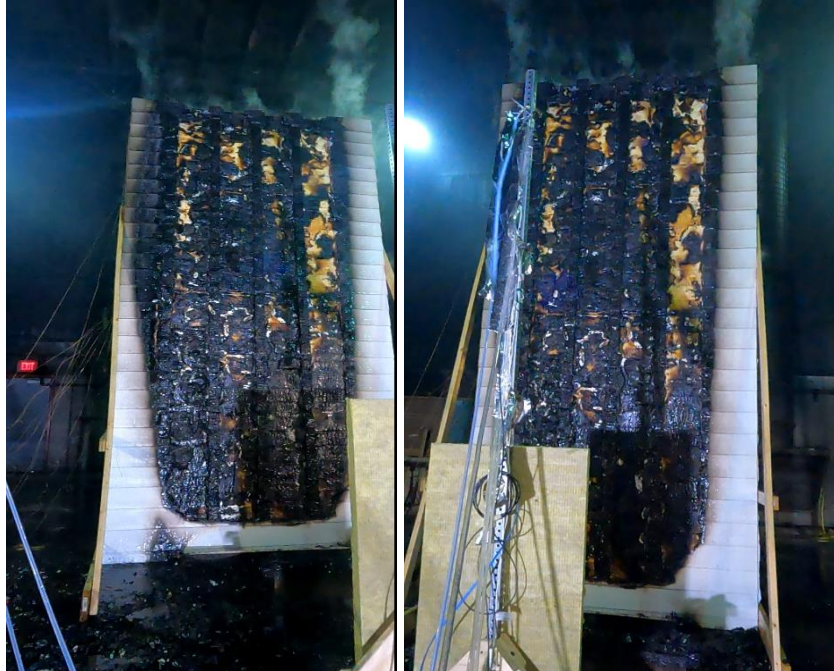
Figure 29 - Post-test Photographs of Test 10 Wood Composite Siding/Furring Strips/Foil Polyiso Wall Assembly with 75 kW Ignition
