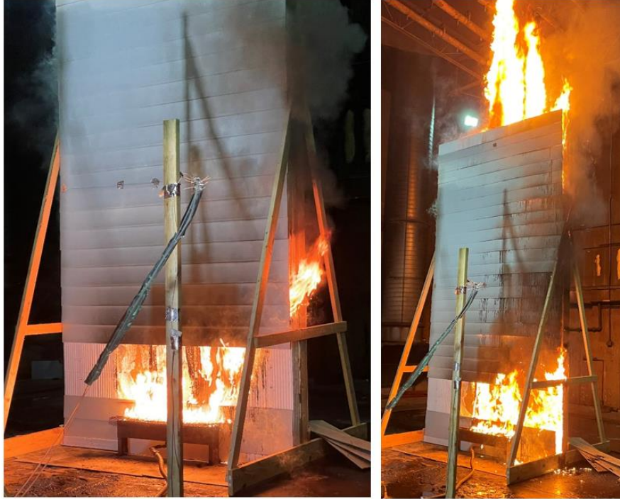
Figure 36 - Photograph of Test 7 with Fiber Cement Siding Panels Removed Showing Interior Fire Spread
