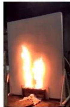
Figure 10. 10. Exp. 26 - Stucco Siding
