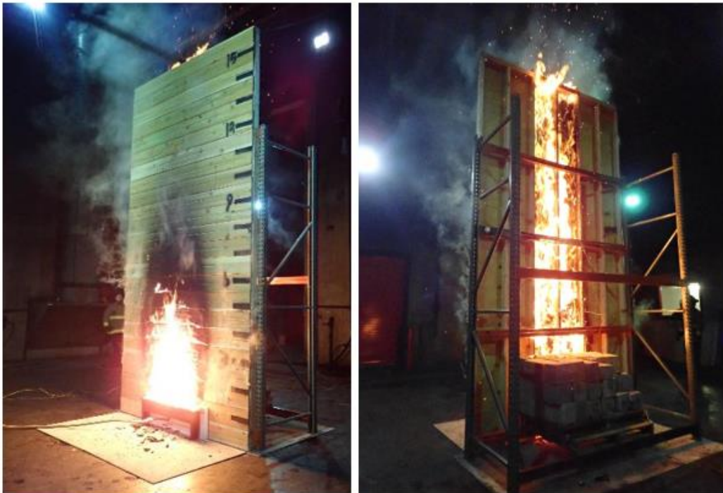
Figure 12 - Photographs of Fire Burning through Test Sample
