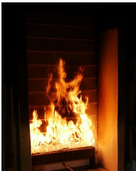
Figure 3 - Photograph of ASTM E2707 Test
