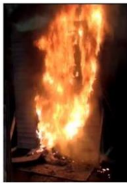
Figure 10. 6. Exp. 5 – Vinyl siding over polystyrene
