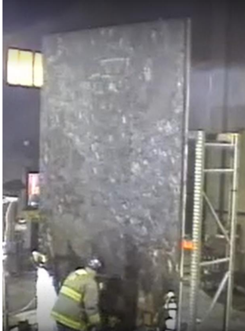
Figure 41 - Post-test Photograph of Test 2 Vinyl Siding/Construction Paper/OSB Wall Assembly with 40 kW Ignition
