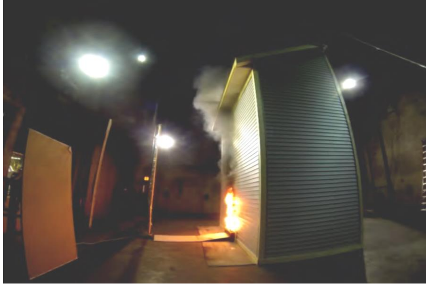
Figure 5 - Photograph of FSRI Eave Experiment [7]
