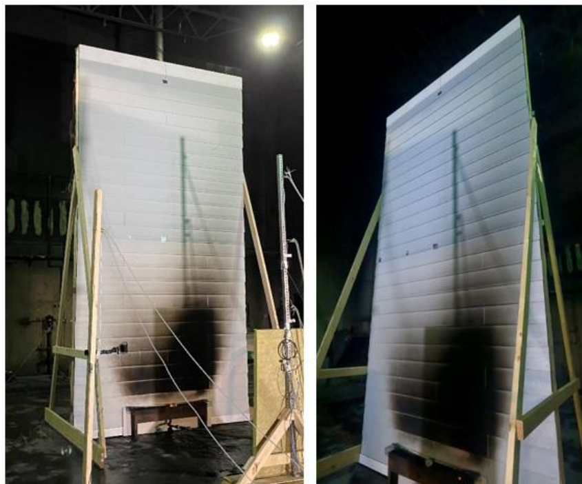
Figure 21 - Post-test Photographs of Test 3 Vinyl Siding/Asphalt Paper Wall Assembly with 75 kW Ignition
