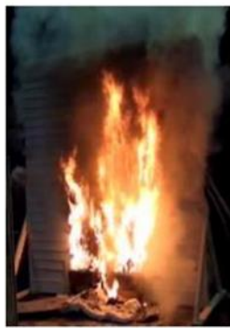
Figure 10. 5. Exp. 3 – Vinyl Siding over plywood
