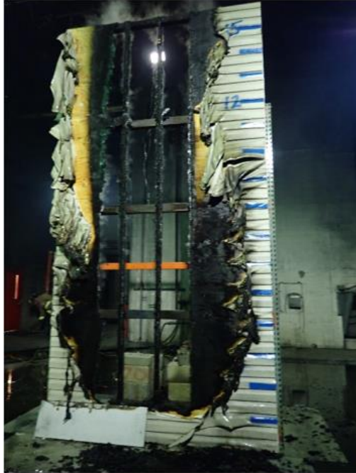
Figure 47 - Post-test Photograph of Test 8 Vinyl Siding/House Wrap/Plywood Wall Assembly with 75 kW Ignition
