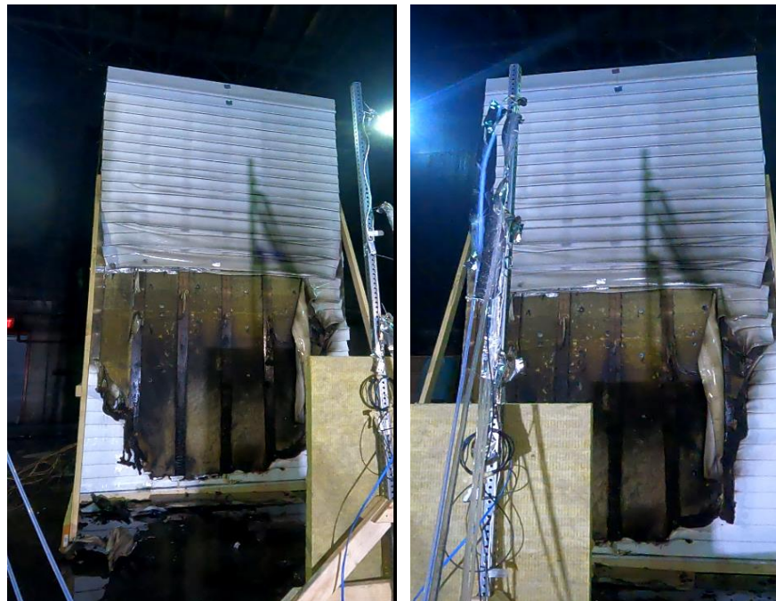
Figure 30 - Post-test Photographs of Test 11 Vinyl Siding/Furring Strips/Mineral Wool Wall Assembly with 75 kW Ignition
