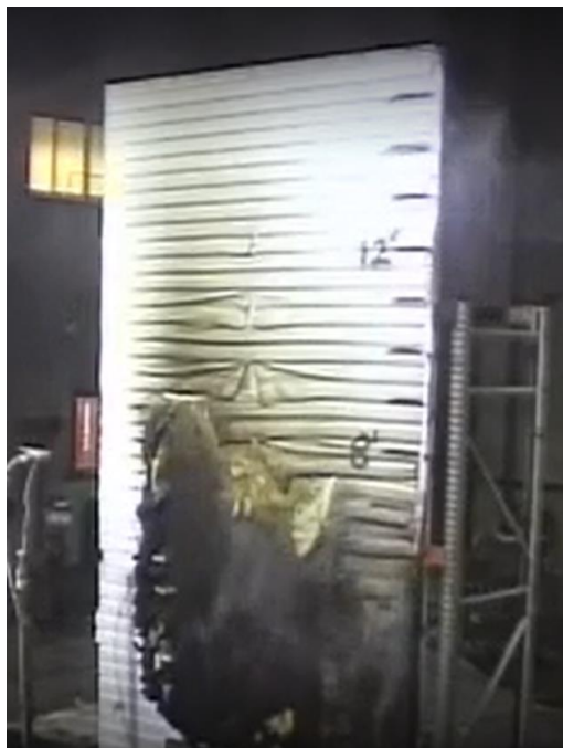
Figure 42 - Post-test Photograph of Test 3 Vinyl Siding/House Wrap/OSB Wall Assembly with 25 kW Ignition
