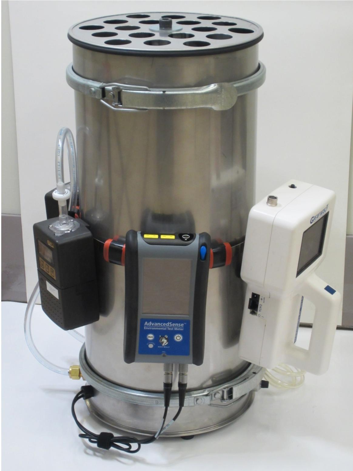
Figure 10. A battery-powered data acquisition system was also mounted on the outside of the cylinder.
