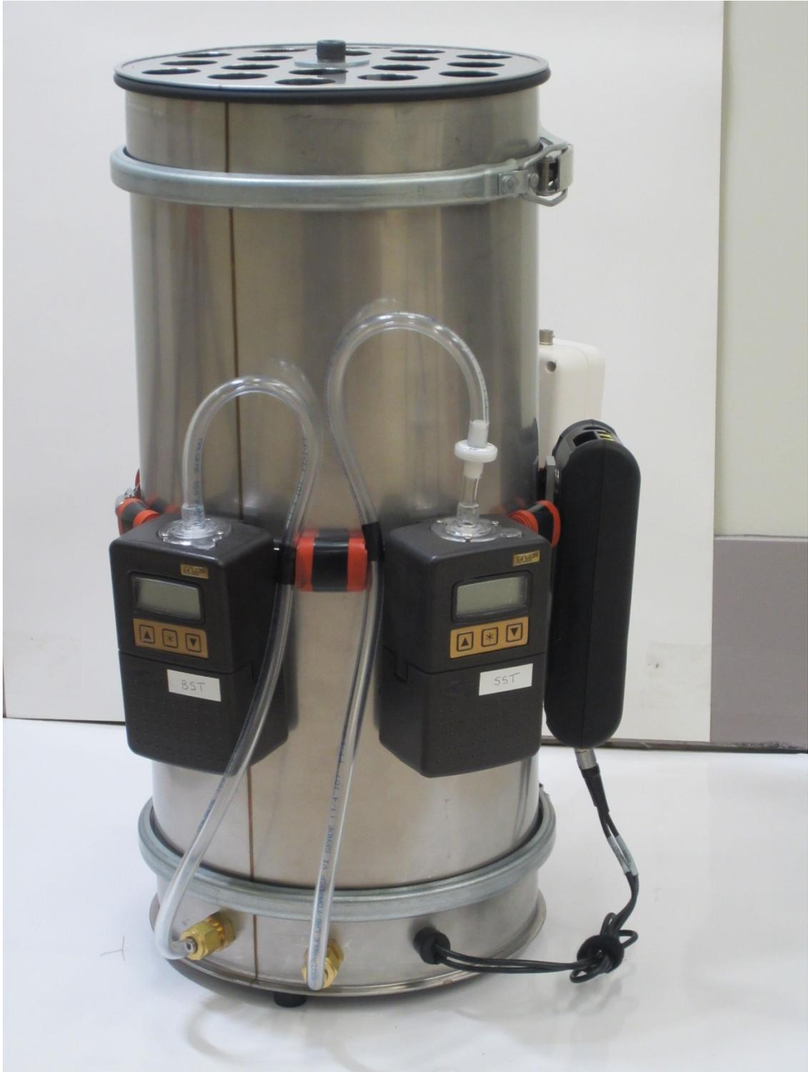
Figure 8. Portable battery-powered pumps are mounted on the outside of the cylinder.
