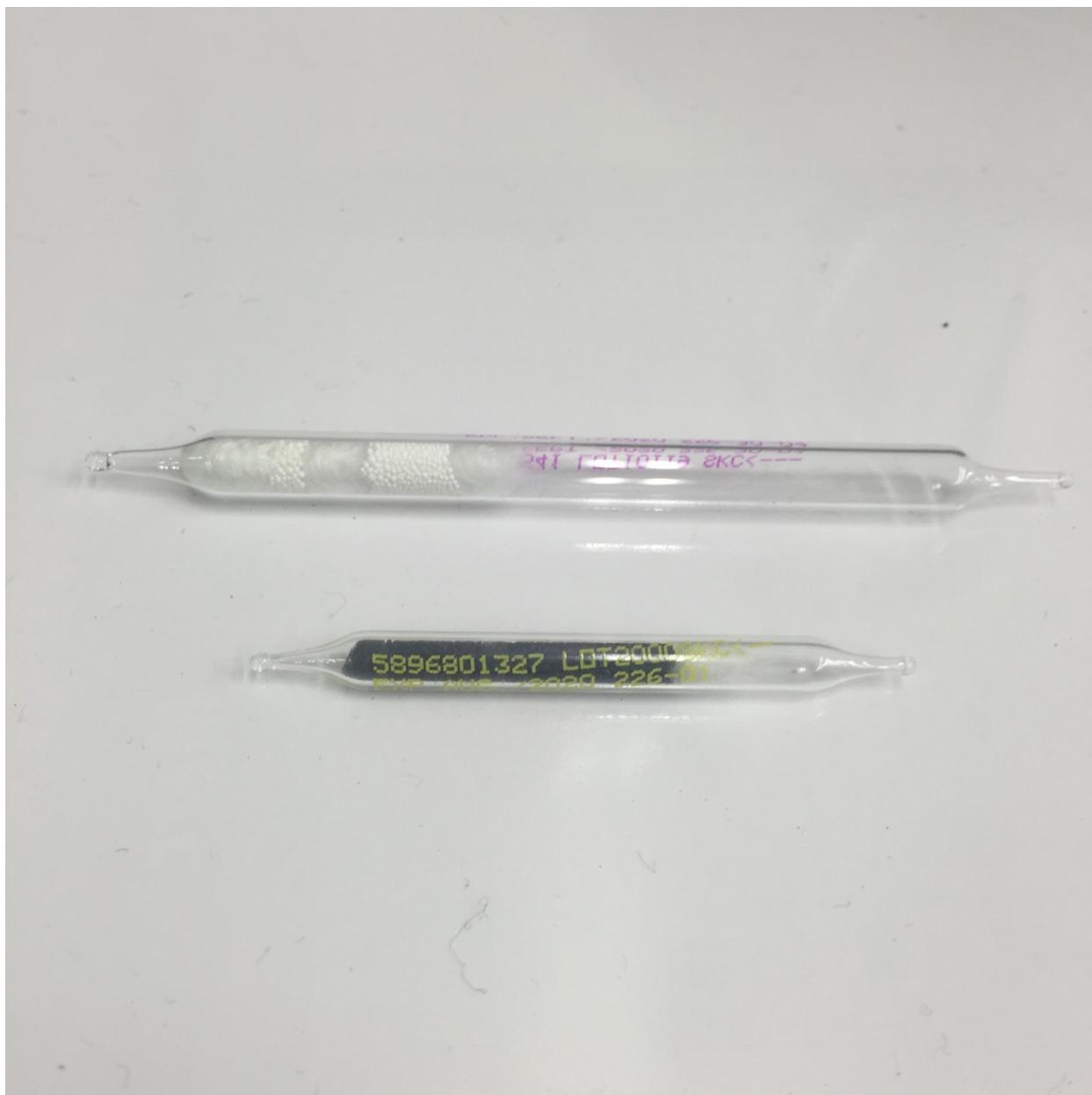
*Figure 7. Sorbent tubes for polycyclic aromatic hydrocarbons (top) and benzene (bottom).*
