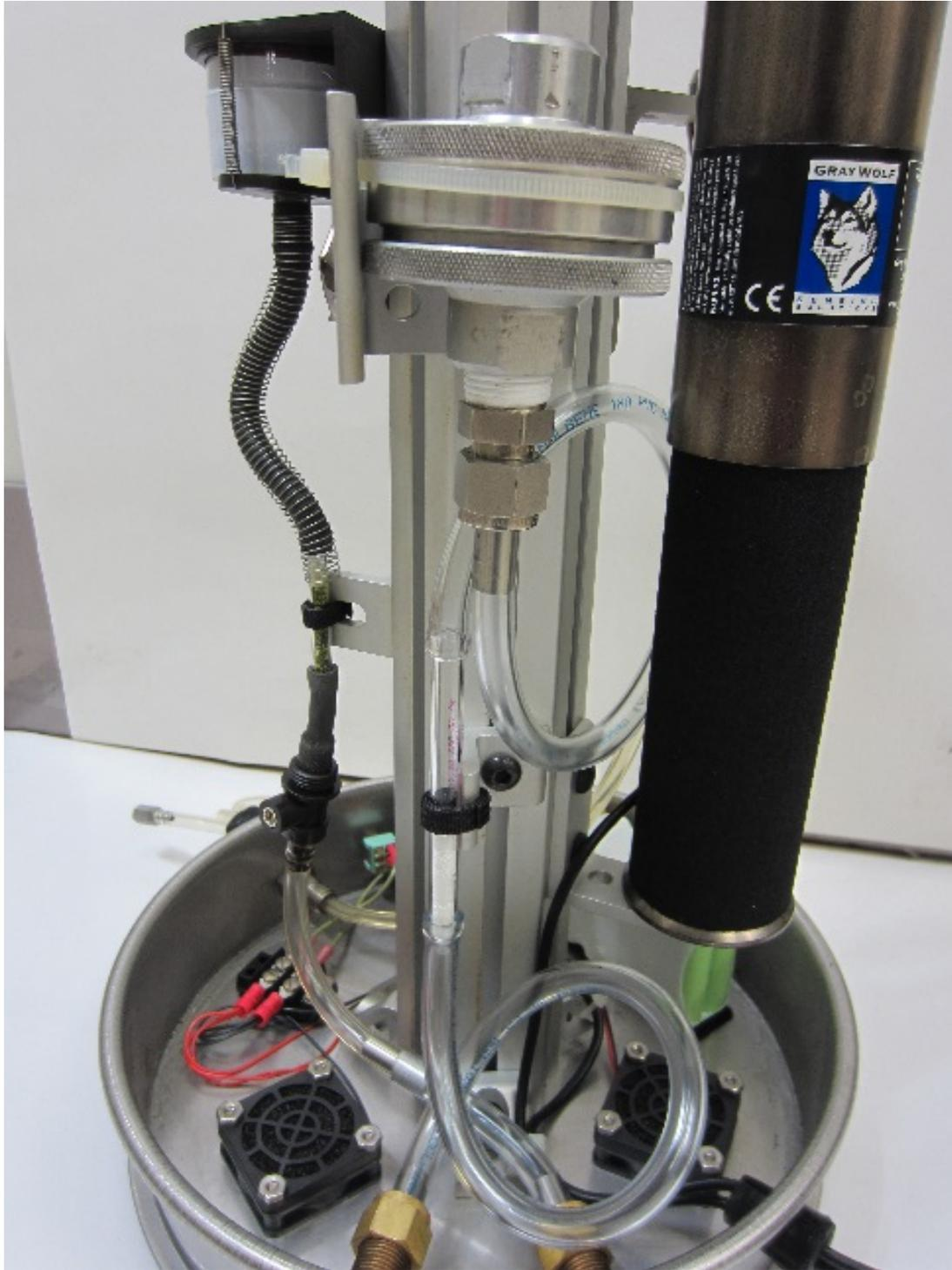
*Figure 6. Sorbent tubes for benzene and polycyclic aromatic hydrocarbons (PAH) are mounted on the opposite side from the multi-gas analyzers.*
