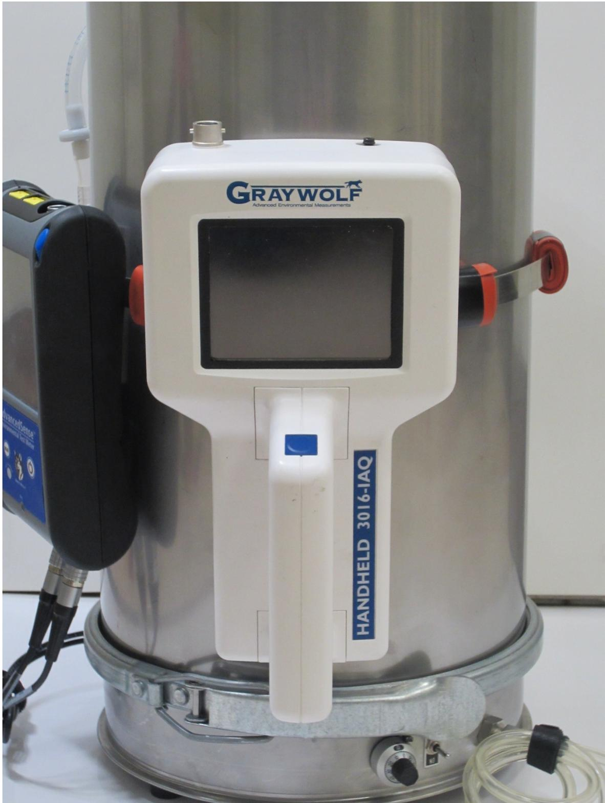
Figure 9. Battery-powered particulate sizing analyzer is also mounted on the outside of the cylinder.
