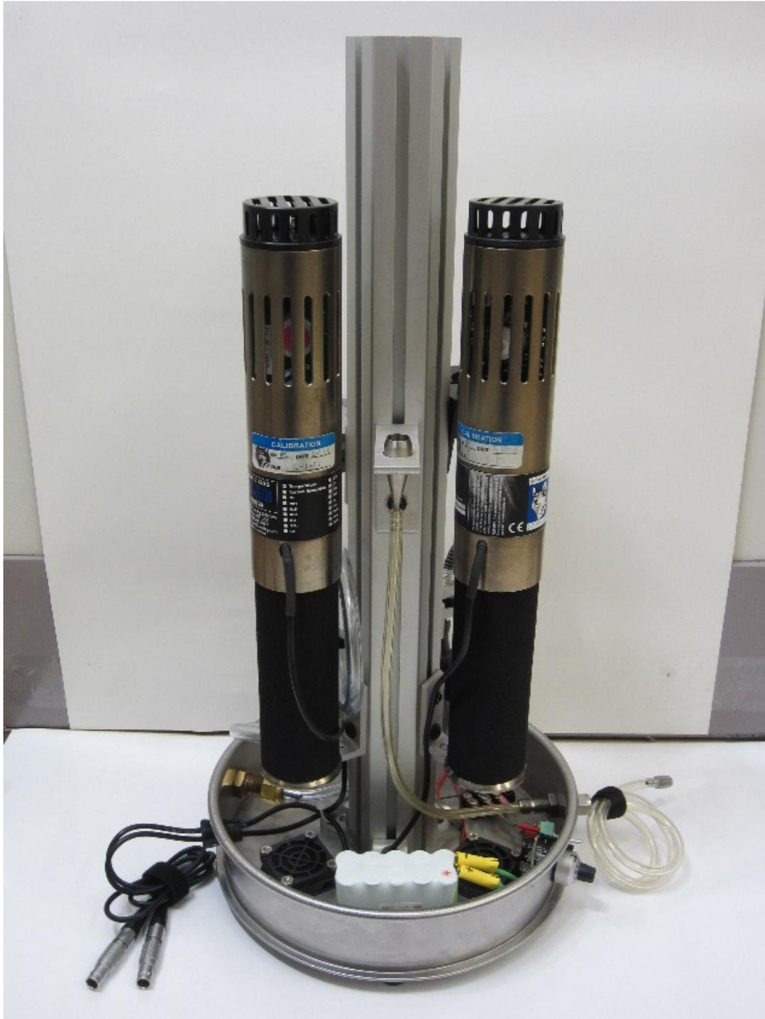
*Figure 4. Multi-gas systems 1 and 2 are positioned parallel to and mounted to the center support. Impact of Ventilation*
