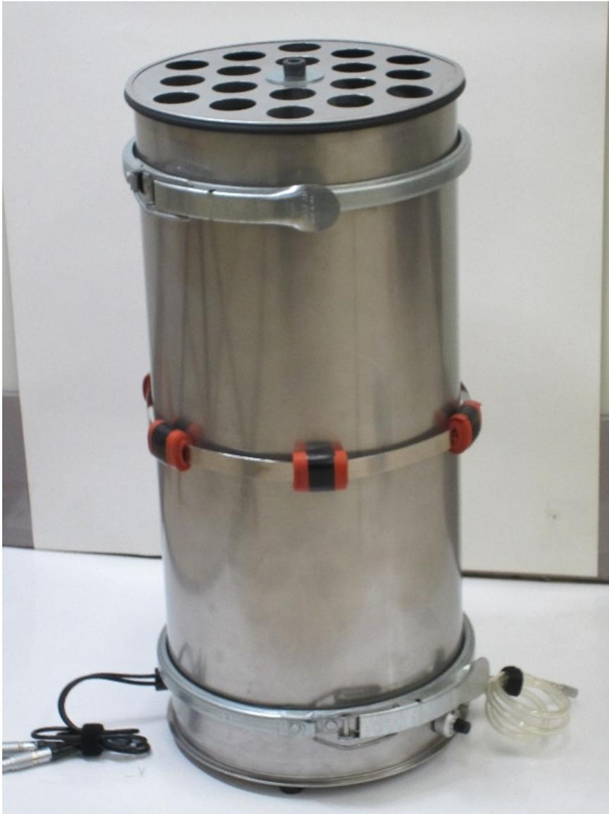
*Figure 1. Stainless steel duct analyzer enclosure.*
