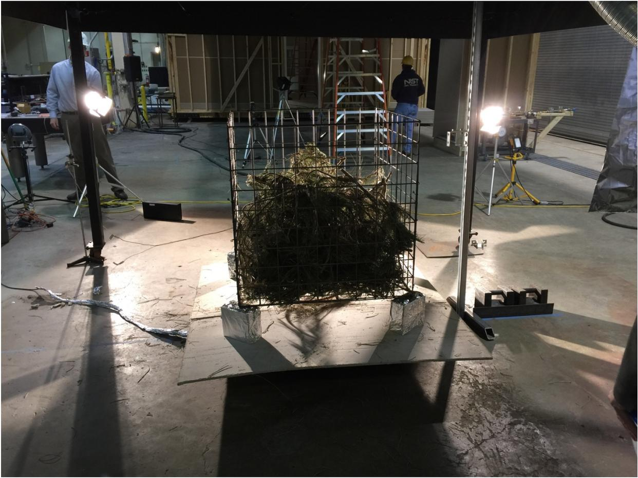
*Figure 12. Weighing the plant material placed into metal cage.*
