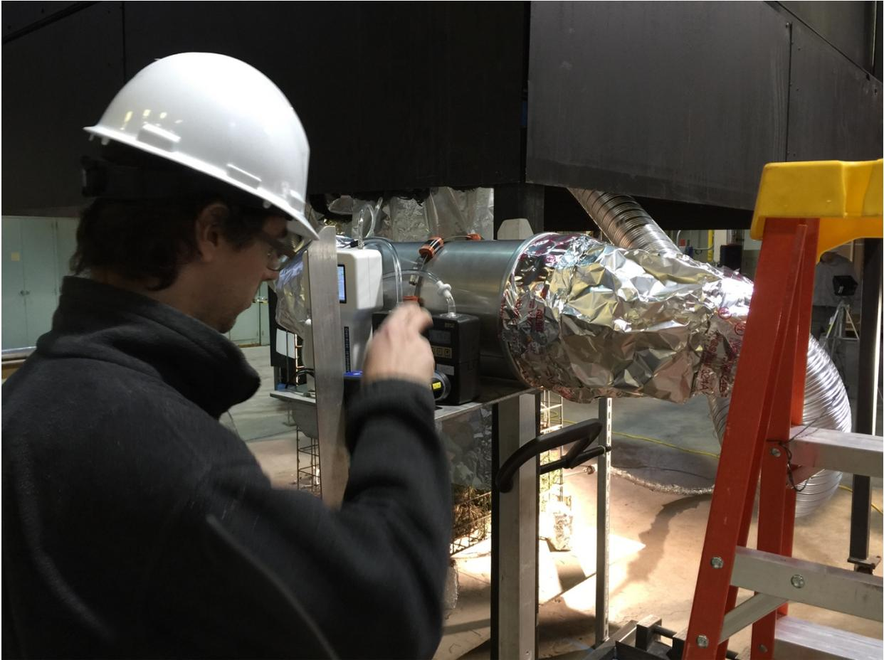
*Figure 14. Sensor platform connected to metal tubes that send smoke through to be analyzed.*
