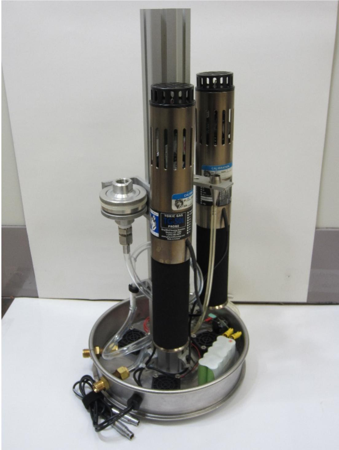
*Figure 5. Filter holder for gravimetric soot mass concentration and small tip for soot particle size analyzer are mounted in between the multi-gas systems*
