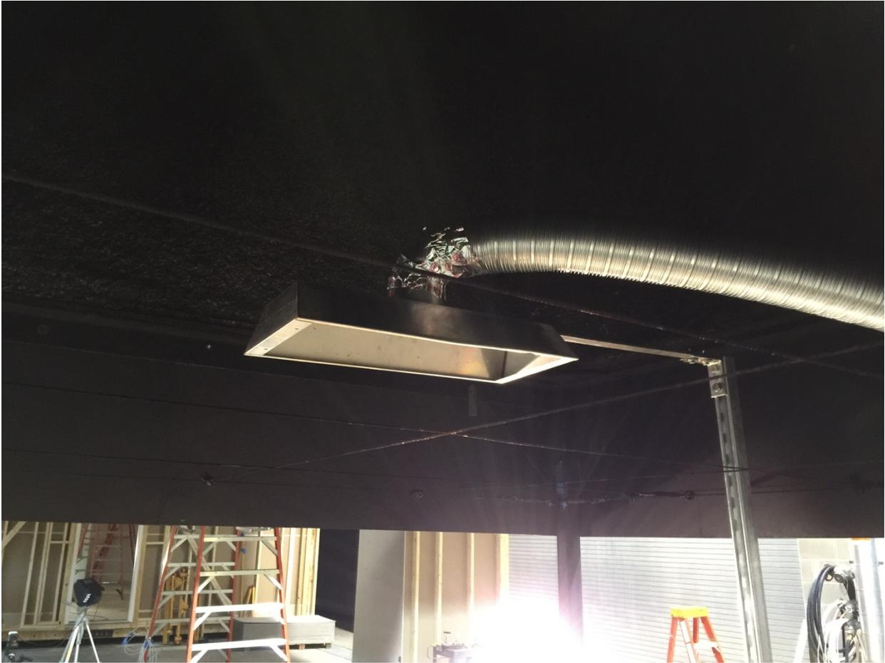
*Figure 13. Metal hood used to collect smoke from the burn, and funnel it to the sensor array.*
