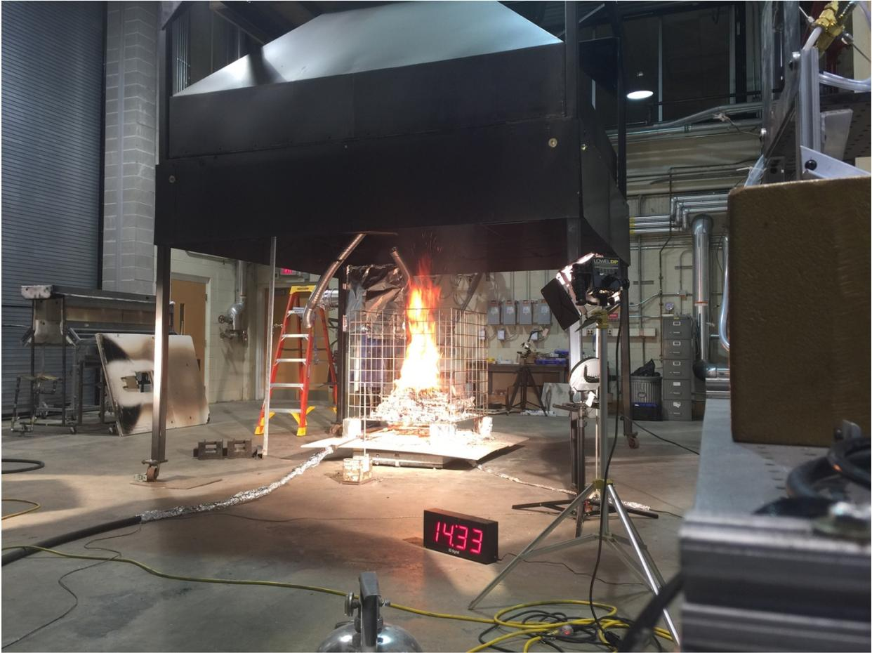
Figure 16. Active burning of pine, gypsum, and PVC to simulate a WUI fire.
