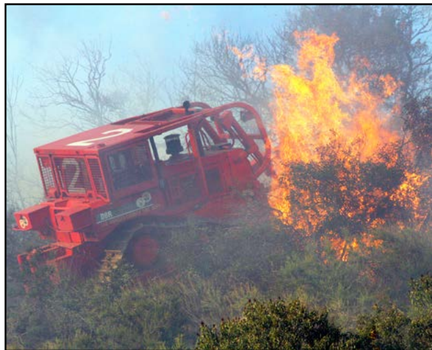
Figure 6.11. Dozers are best suited for direct and indirect control line construction over long distances.
