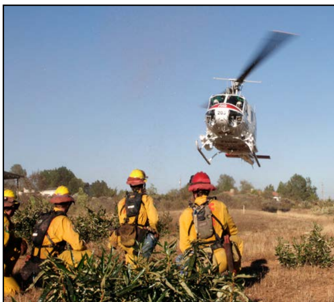
Figure 10.29. Rotor wash from helicopters can propel small rocks, sticks and other projectiles in all directions, and dislodge fire weakened trees.
