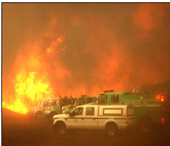
Figure 10.39. Entrapment avoidance means planning for what COULD happen by parking equipment in safe areas for temporary shelter or escape.
