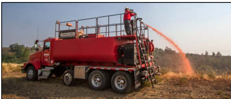
Figure 6.29. Long term retardants can be effectively applied from ground based platforms allowing for greater flexibility when choosing application sites.
