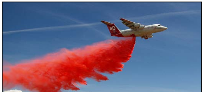
Figure 6.23. The BAE 146 Type 1 airtanker carries a minimum payload of 3,000 gallons. The legacy BAE 146 is a Type 2 airtanker which carries a minimum payload of 1,800 gallons.
