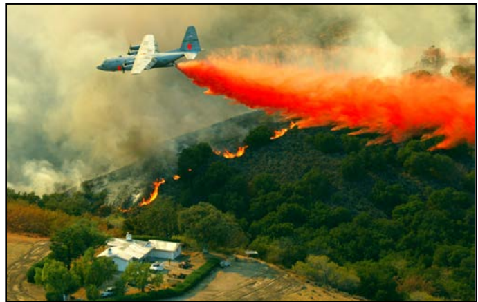
Figure 6.26. MAFFS (Modular Airborne Fire Fighting System) are National Guard assets that are deployed during periods of significant fire activity. They are a Type 1 air tanker carrying 3,000 gallons of retardant.
