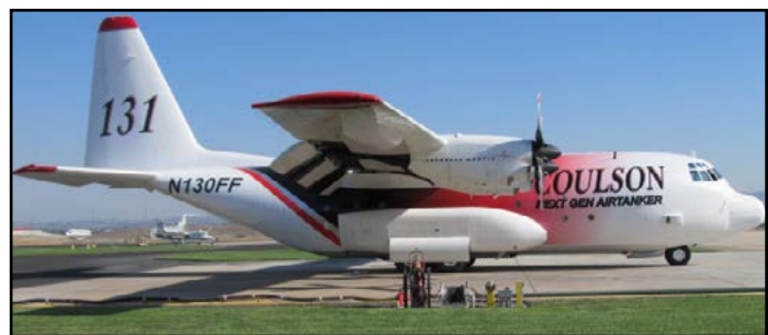
Figure 6.24. The C-130Q is one of the new generation air tankers. It is a Type 1 airtanker carrying a payload of 3,000 gallons of retardant with a constant flow tank.
