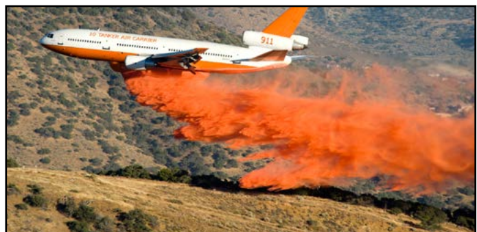
Figure 6.27. VLATs are capable of dropping very large amounts of retardant over a wide area.
