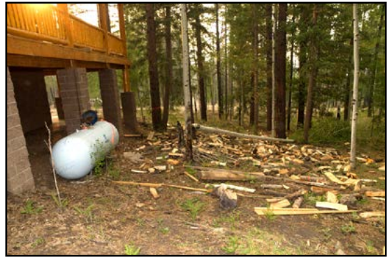
Figure 4.8. The evaluation of the fuel component in the WUI should include wildland fuels, ornamental vegetation, wood piles, propane and other fuel tanks, their proximity to the structure and the structure itself as part of the fuel load. Photo courtesy of Kari Greer.
