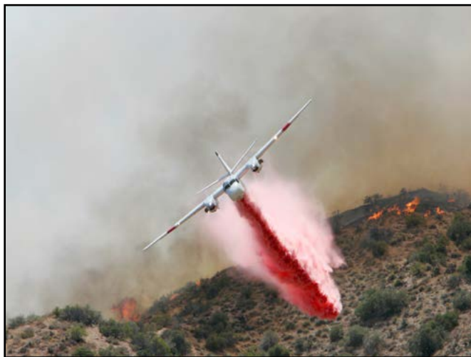
Figure 10.28. Avoid serious injury by getting out of the drop zone. If a direct hit is unavoidable, immediately assume a position on the ground facing the aircraft securing tools and hard hats.
