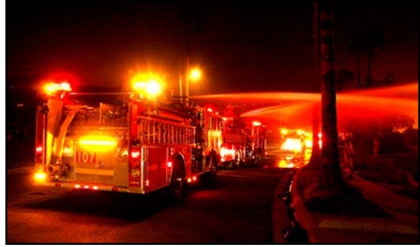
Figure 5.29. Anchor and Hold resources should consider using master stream devices to flow large volumes of water in an effort to defend exposures and to suppress fully involved structures thus reducing ember production.
