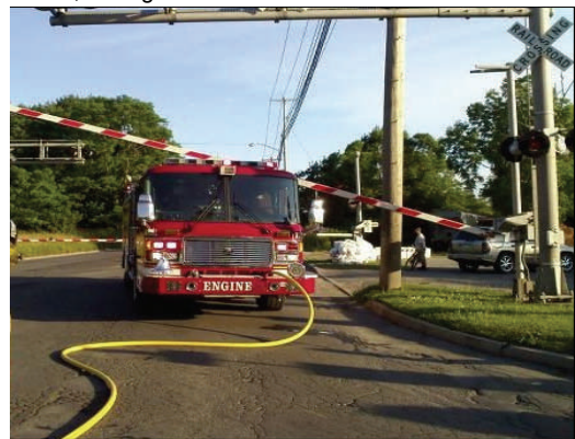
In a separate incident, in another state, this engine was operating at a car fire. The engine did not clear the crossing gates. Luckily, the freight train saw the rear lights on the engine, and was traveling slow enough so it could stop in time.
