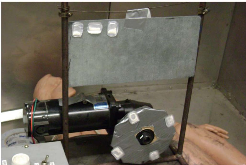
Figure 13 – Placement of PADs for Exposure Condition Experiments
