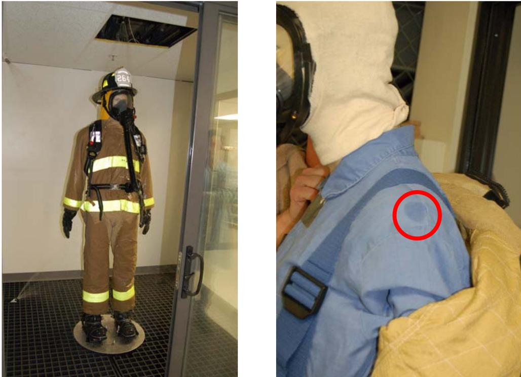
(a) Overall Shower Test Set Up      (b) Water Mark on Right Shoulder
